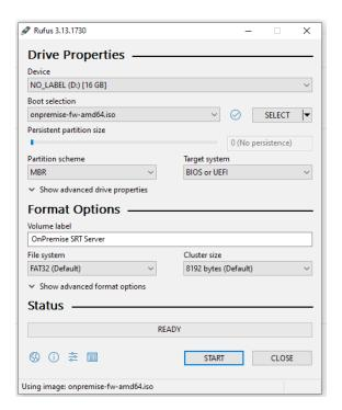
Choose Write in DD Image mode, and accept the warning of data destroyed.
